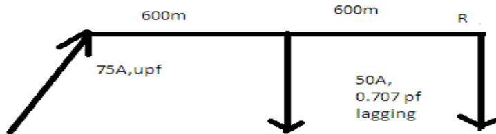
54. A single phase distributor PQR fed at P is as shown in figure. The power factors are lagging and expressed relative to the voltage at the far end is 230V. calculate the voltage at the supply end and its phase angle with respect to the far end.
