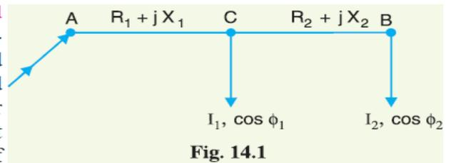
$$\text{Impedance of section } AC, \quad \overline{Z}_{AC} = R_1 + j X_1$$
