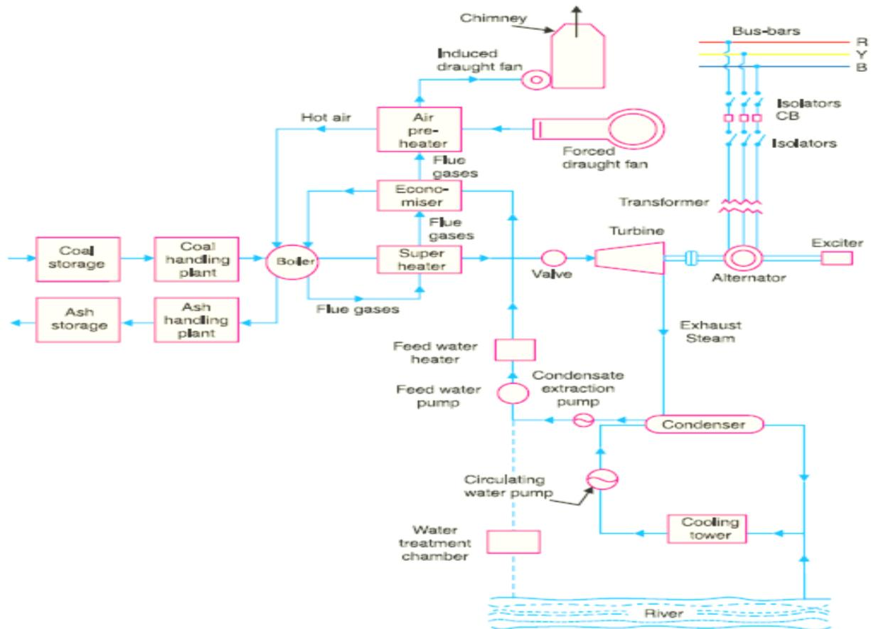
Although steam power station, simply involves the conversion of heat of coal conversion into electrical energy, yet it embraces many arrangements of proper working an efficiency.
