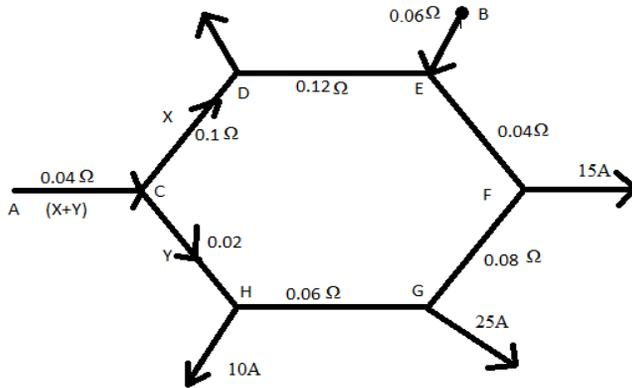
39. Figure shown in a ring distributor with interconnector BD. The supply is given at a point A. the resistance of go and return of various sections are indicated in the figure. calculate
