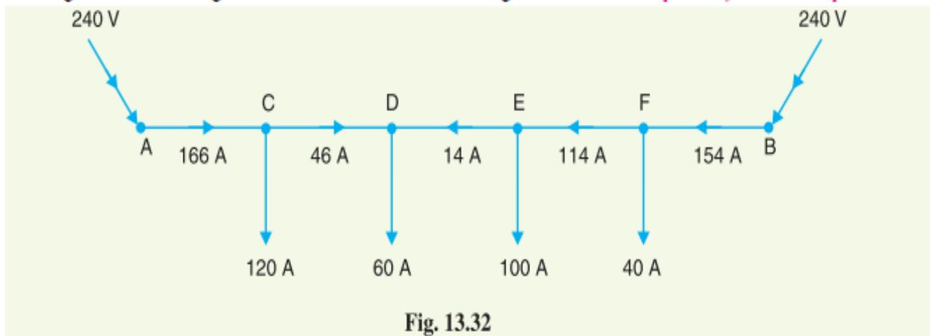
**(ii)** The feeding point A will supply 166 A due to concentrated loading plus  $0.5 \times 400 = 200 \text{ A}$  due to uniform loading.
