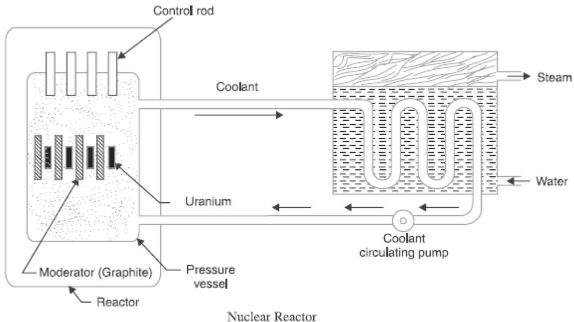
(ii) Heat exchanger: The coolant gives up heat to the heat exchanger which is utilized in raising the steam. After giving up heat, the coolant is again fed to the reactor.
