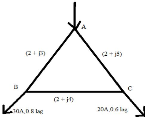
61. A 3-phase, 6.6 KV sub-station supplies a load of 120A at 0.8 p.f lagging at B and 75A 0.6 p.f lagging at C. the impedance of each branch is shown in figure. Find out the current in each branch, the p.f of load are referred to the section A.
