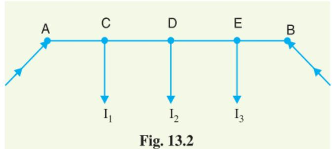
on decreasing as we move away from one feeding point *say*  $A$ , reaches minimum value and then again starts rising and reaches maximum value when we reach the other feeding point  $B$ . The minimum voltage occurs at some load point and is never fixed. It is shifted with the variation of load on different sections of the distributor.
