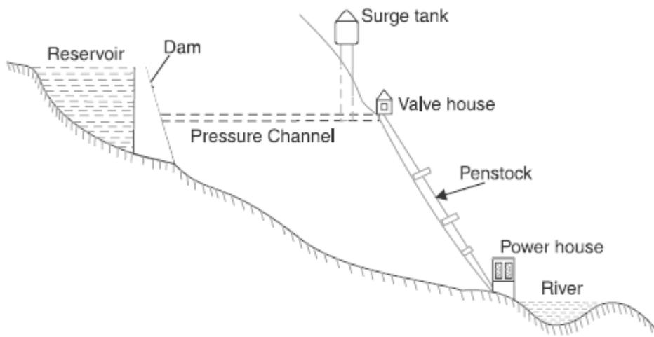
Schematic arrangement of a Hydro-electric plant
