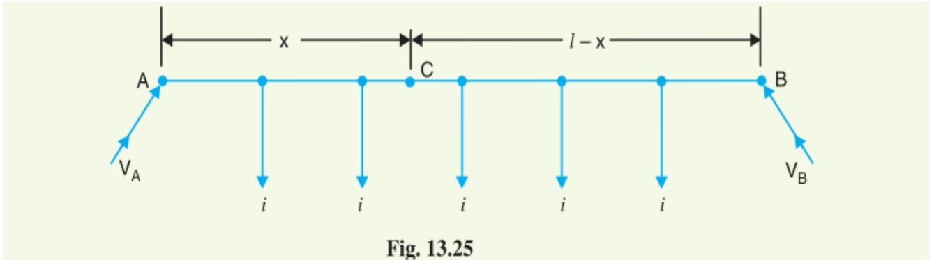
As the distance of C from feeding point B is  $(l-x)$ , therefore, current fed from B is  $i(l-x)$ .
